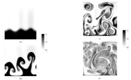
Fig. 3. Computed temperature values for the high Rayleigh number convection problem at times 1(a), 2.5(b), 4(c) and 5.5(d)
