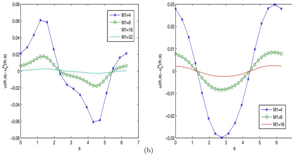
Fig. 4.1. The errors on artificial boundary for with different mesh sizes. (a): Example 1 with  $N = 10$ ; (b): Example 2 with  $N = 5$ .
