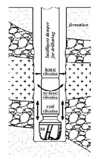
Figure 1: Bottom hole assembly (BHA) and vibration modes.
