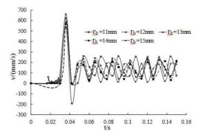
Figure 14: Effect of ball diameter on its kinematics characteristics.
