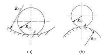
Figure 11: Principal plane of mandrel (through contact point A).
