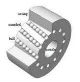
Figure 3: Vibration converter model.
