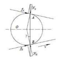
Figure 9: Schematic diagram of self-locking effect.
