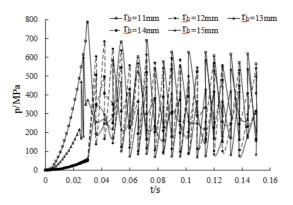
Figure 16: Effect of ball diameter on its contact stress.
