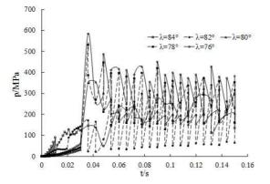
Figure 17: Effect of helix angle on contact stress of ball.
