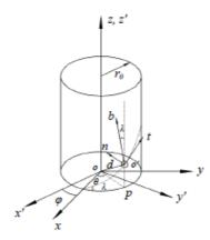
Figure 5: The position of the ball center, o', in the Cartesian coordinates and Frenet coordinate.
