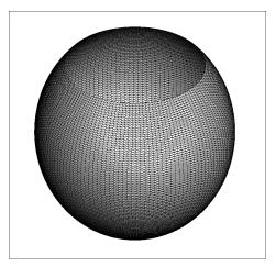
Fig. 7.6. Mesh (hollow35) of the hollow sphere of radius 1m. The interface (not represented) possesses 7420 DoF while the whole sphere has 44100 DoF.
