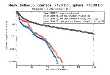
Fig. 7.9. Convergence curves to reach a residue of order  $10^{-4}$ , for the mesh hollow35 of the hollow sphere, whose interface is meshed with 7420 DoF, at a frequency of 1 GHz, respectively for DDM Y0 (unpreconditioned) and DDM Y1, DDM Y2, DDM Y3 (with analytic preconditioners).
