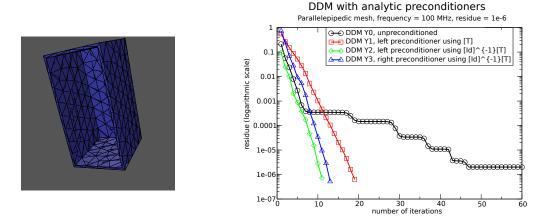
Fig. 7.2. Mesh (left) and convergence curves (right) to reach a residue of order  $10^{-6}$ , for the parallelepipedic box at 100 MHz meshed with 102 DoF on the interface  $\Sigma$ .
