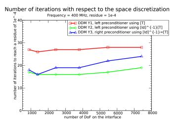
Fig. 7.8. Comparison of the number of iterations for the preconditioned equations DDM Y1, DDM Y2, DDM Y3, to reach a residue of  $10^{-4}$ , at a constant frequency of 400 MHz. For each curve, each point corresponds to one of the different meshes that we have considered, namely with 888, 1380, 2440, 3800, 5460 and 7420 DoF on the interface.
