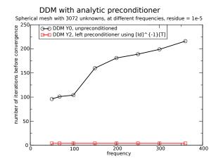
Fig. 7.4. Mesh (left) and influence of the frequency increase (right) on the number of iterations to reach a residue of order  $10^{-5}$ , for the artificial sphere meshed with 3072 DoF.
