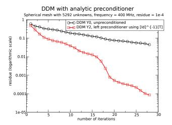
Fig. 7.5. Convergence curves to reach a residue of order  $10^{-4}$ , for the spherical mesh with 5292 DoF, at a frequency of 400 MHz, respectively for DDM Y0 (unpreconditioned) and for DDM Y2 (with analytic preconditioner).
