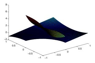
Fig. 3.4. Interface cuts one Vertex of a Triangle.
