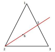
Fig. 2.5. The interface comes across one vertex and one edge of the triangle.
