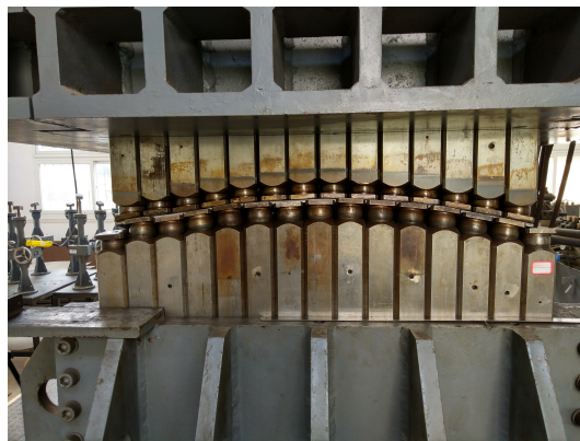
Figure 1: Multi-square punch forming (MSPF) by SKWB-400.
