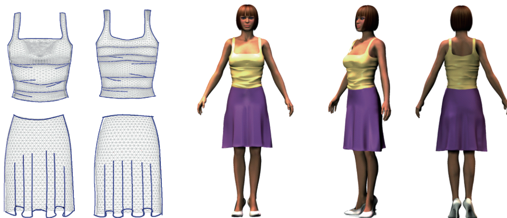
Fig. 1: 3D virtual garments generation based on surface deformation. Left: digitalized designer's sketches. Right: resulting 3D garment model.
